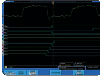
► Multi-channel setup-and-hold triggering highlighting multiple violations (MSO4000).
