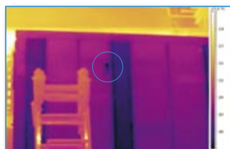
◆ IR image shows thermal bridges and a moisture spot in the insulation
