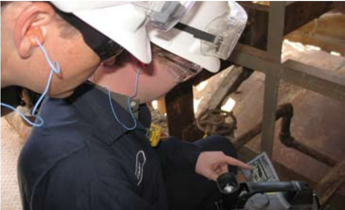
Co-workers identify the location of a gas leak
