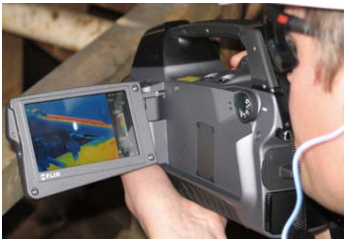
Real-time image of the gas cloud displayed on the built in LCD screen
