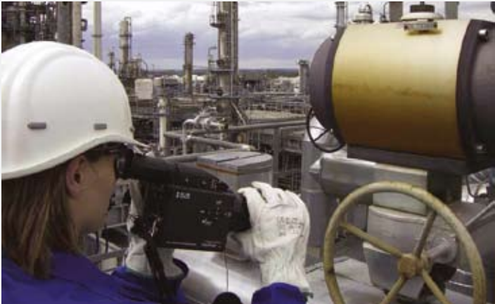
Examining potential leak paths
